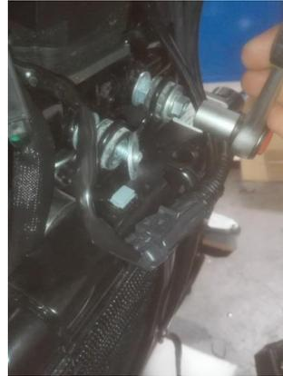
6. Insert the rubber fixings into the lower bracket.
